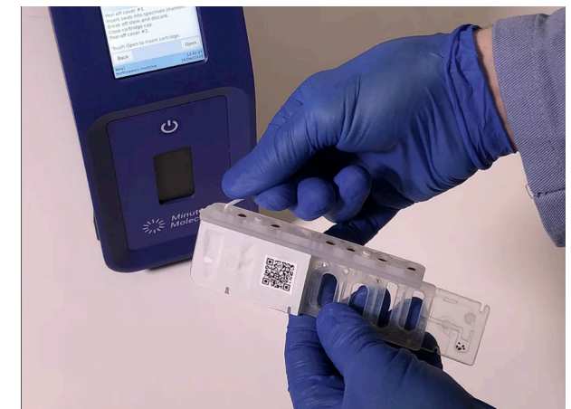
DASH (Diagnostic Analyzer for Specific Hybridization) Photo courtesy of Minute Molecular Diagnostics
